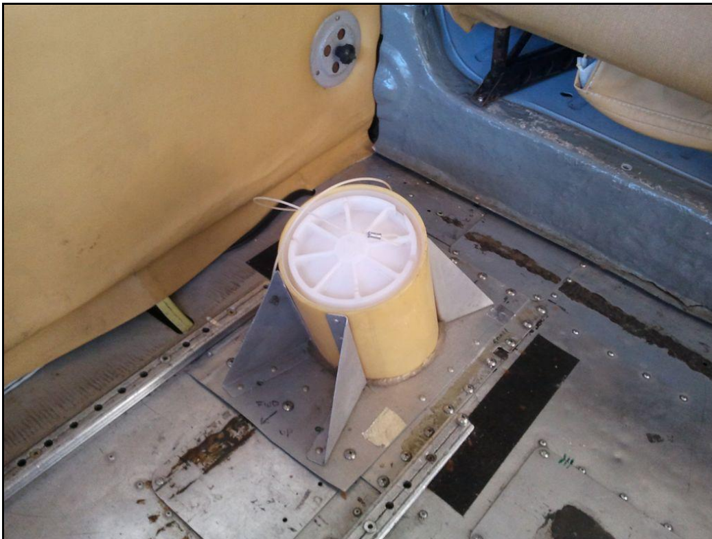
Photo 1. View of sonobuoy chute from inside the Partenavia aircraft. The white disk is a cover that keeps the wind from blowing inside the aircraft, and is removed immediately prior to sonobuoy launch.
